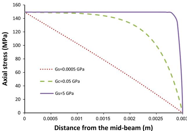
Fig. 9. Axial stress of the core fibre against the distance measured from the mid-beam ( $z = 0$ ) with different shear modulus of the sericin.
