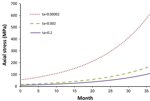
Fig. 14. Axial stress between the sericin and the core fibre calculated from (a) the increase in moisture content based on time with different thickness of the sericin.
