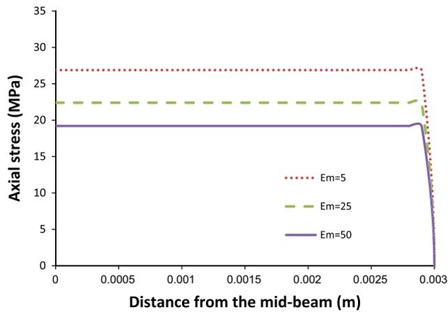
Fig. 8. Axial stress of the core fibre against the distance measured from the mid-beam ( $z = 0$ ) with different Young's modulus of the host polymer material.
