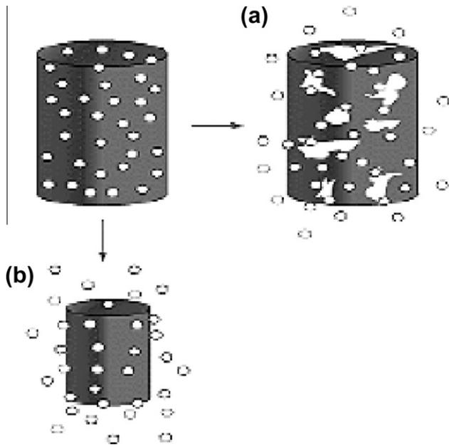
Fig. 12. The scheme of (a) bulk erosion and (b) surface erosion [1].
