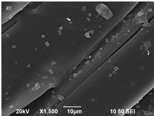
Fig. 1. Micrometre-sized calcium oxalate crystals on the surface of tussah silk fibre.
