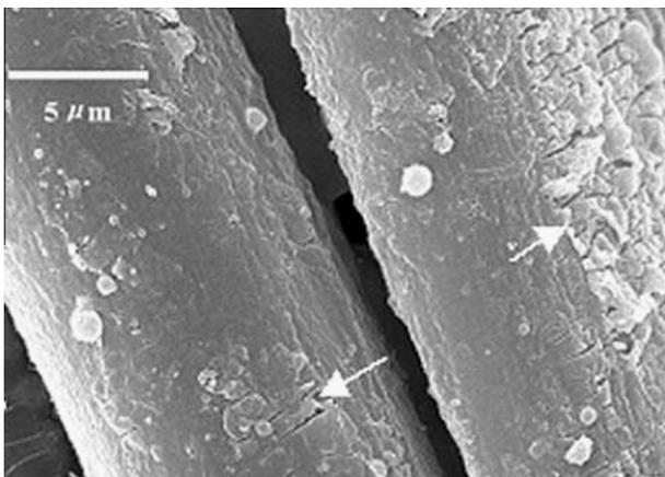
Fig. 4. Scanning electron micrographs illustrating silk fibre degummed by succinic acid [61].
