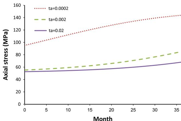
Fig. 17. The effect of the moisture content of host polymer material and core fibre on the axial stress in the fibre depending on time.
