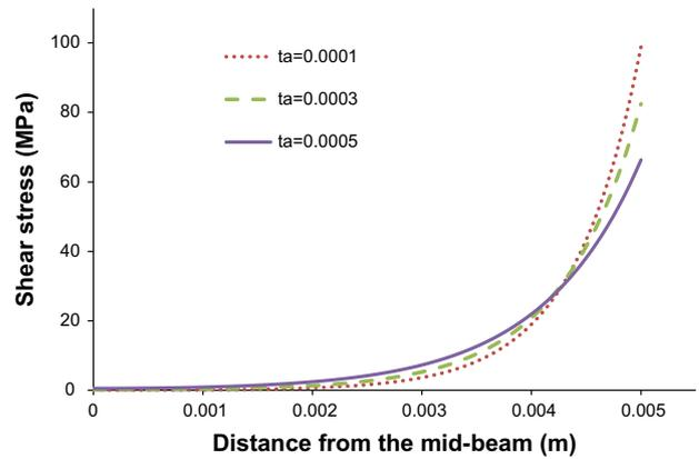
Fig. 11. Shear stress of the core fibre against the distance measured from the mid-beam ( $z = 0$ ) with different thickness of sericin.
