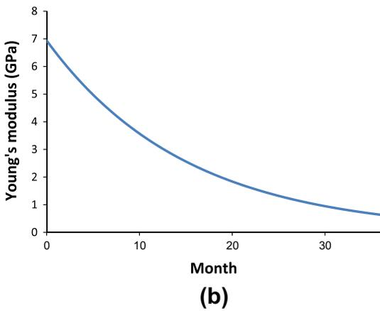
Fig. 13. The Young's modulus of host polymer material calculated from (a) the change of moisture content and (b) time.
