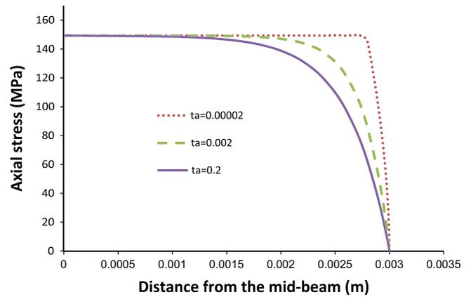
Fig. 10. Axial stress of the core fibre against the distance measured from the mid-beam ( $z = 0$ ) with different thickness of sericin.
