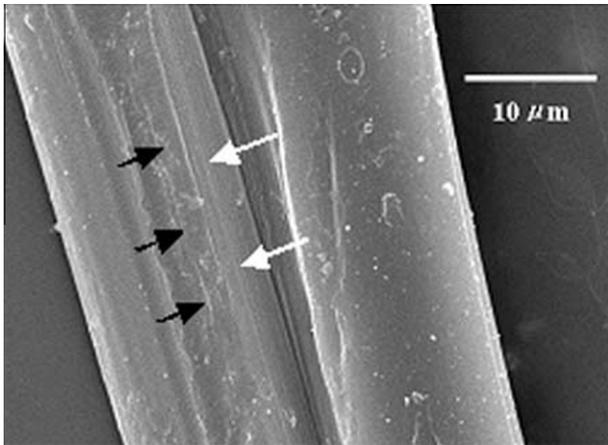
Fig. 3. Surface of *Bombyx mori* silk fibre degummed by  $\text{Na}_2\text{CO}_3$  [61].
