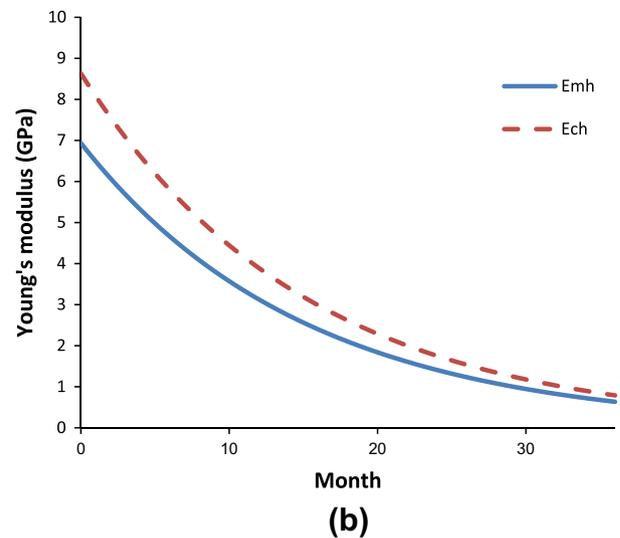
Fig. 16. The Young's modulus of host polymer material and core fibre measured from (a) the change of moisture content of host polymer material and (b) time.
