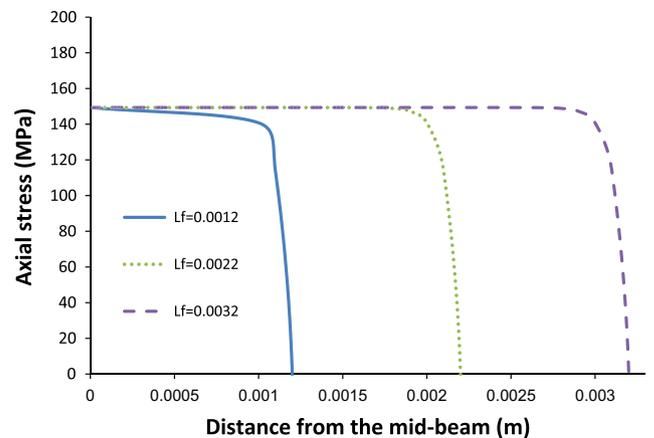
Fig. 6. Axial stress of the core fibre against the distance measured from the mid-beam ( $z = 0$ ) with different embedding lengths.
