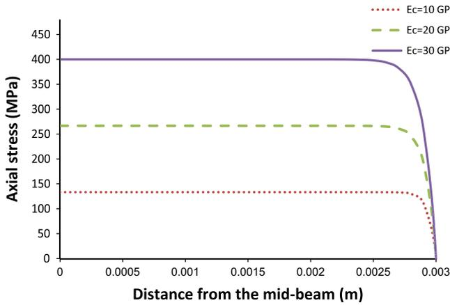
Fig. 7. Axial stress of the core fibre against the distance measured from the mid-beam ( $z = 0$ ) with different Young's modulus of the core fibre.
