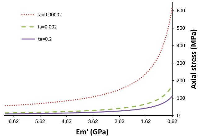
Fig. 15. Axial stress between the sericin and the core fibre calculated from (a) the change of Young's modulus of host polymer material based on the increase in moisture content with different thickness of the sericin.
