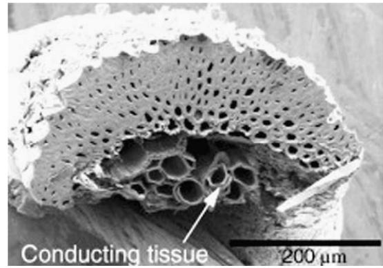
Fig. 2. Hollow section of a sisal fibre [5].
