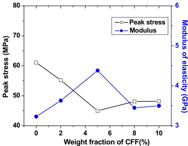
Fig. 7. Relationship between tensile properties and CFF content of CFF/PLA composite.
