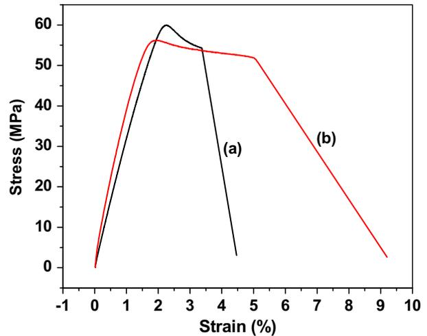
Fig. 8. Stress–strain curves of (a) pure PLA sample; (b) 5 wt% CFF/PLA composite.
