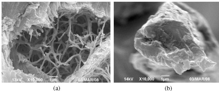
Fig. 5. Flight chicken feather fibre (a) and down chicken feather fibre (b).
