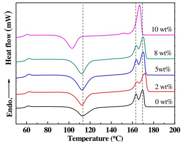
Fig. 9. DSC curves of pure PLA and CFF/PLA composites.
